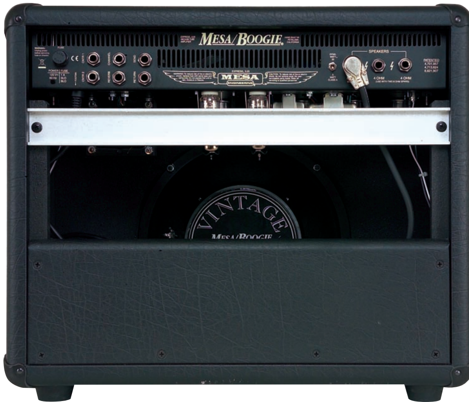
The 5:25's rear panel sports remote switching jacks, an effects loop, and a trio of speaker jacks.
