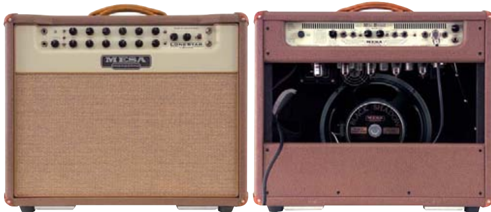
The Lonestar Special's controls can be a little hard to identify unless you're looking straight at the front panel. The tubes are easily accessed without having to remove anything.
