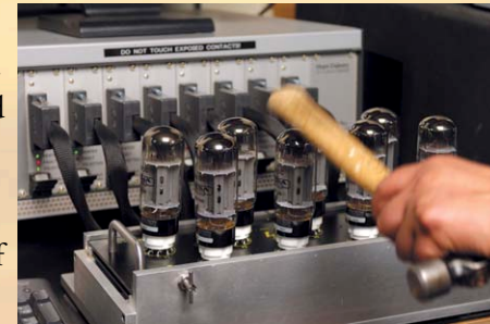
Every tube gets the human hammer test under operating conditions emulating the real life rigours of shock and vibration on the road.
