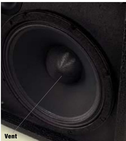
Neodymium speaker magnets can, if not adequately heatsinked and ventilated, lose magnetic strength when subjected to their voice coils' high temperatures. To dissipate heat, the Scout's 12" neodymium driver has heat sinks on the rear motor assembly and is vented through the front, as shown here.
